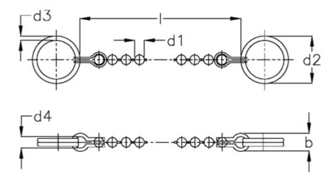
$\begin{array}{lll} b & = 6 \\ d1 & = 3.5 \\ d2 & = 24 \\ d3 & = 1.5 \\ d4 & = 4 \\ I & = 1000 \\ Static load (N) = 100 \end{array}$
